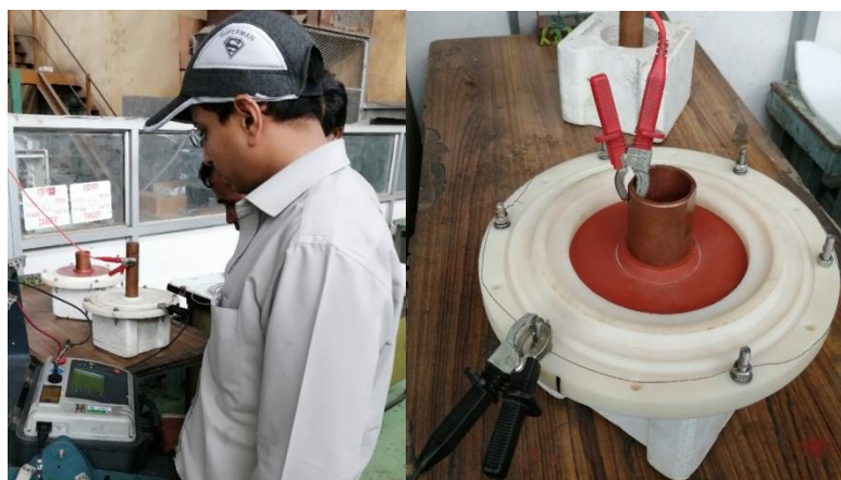
Figure 22: Test set-up for Meggering test
